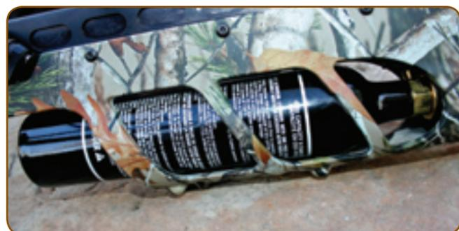
A 9-ounce CO<sub>2</sub> tank screws easily into the bow's stock through the crossbow's open forearm. Depending upon temperature, a tank of CO<sub>2</sub> provides between 40 and 50 cocks/un-cocks.
